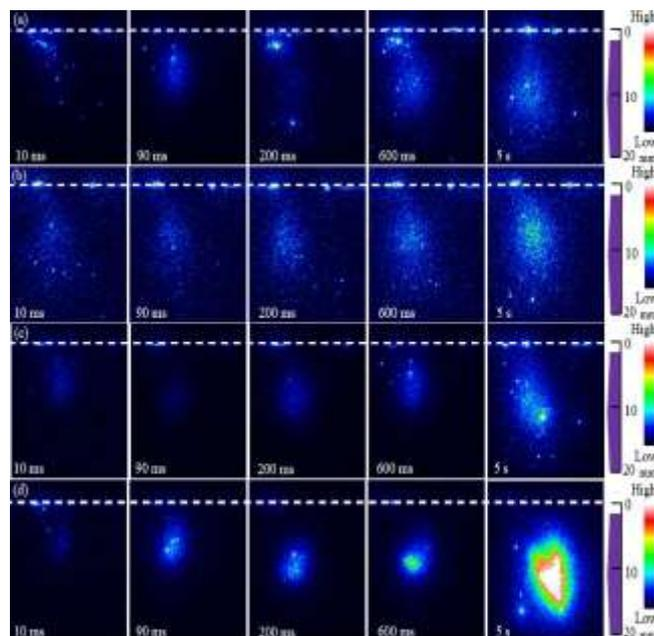
**Fig. 3** Temporal changes of spatial distribution of SiO<sub>2</sub> nanoparticles in Ar gas at (a) 400 Pa, (b) 670 Pa, (c) 1300 Pa and (d) 2700 Pa.
