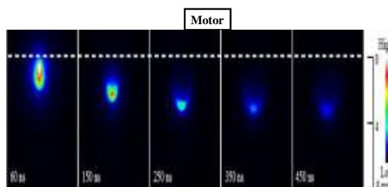
**Fig. 2** Plasma emission image in Ar gas at 400 Pa.
